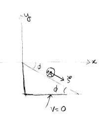
$$L = \frac{1}{2}M\dot{x}^2 + \frac{1}{2}m\left(-\dot{x} + \dot{\xi}\cos\phi\right)^2 + \frac{1}{2}m\dot{\xi}^3\sin\phi + \frac{1}{2}I\dot{\phi}^2 + \frac{1}{2}m\dot{\xi}^3\sin\phi$$
