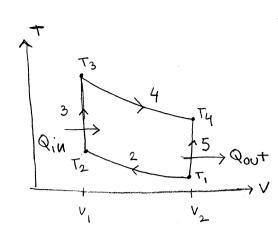
\* otto cycle 15 an Internal combustion enginl
