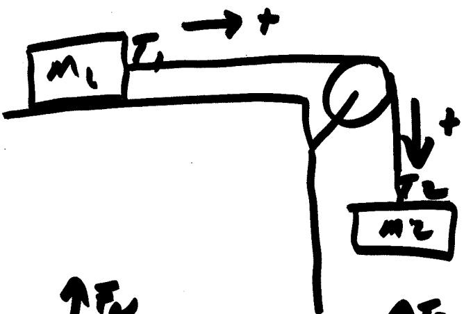
Pulley has moment of inertia  $I$
